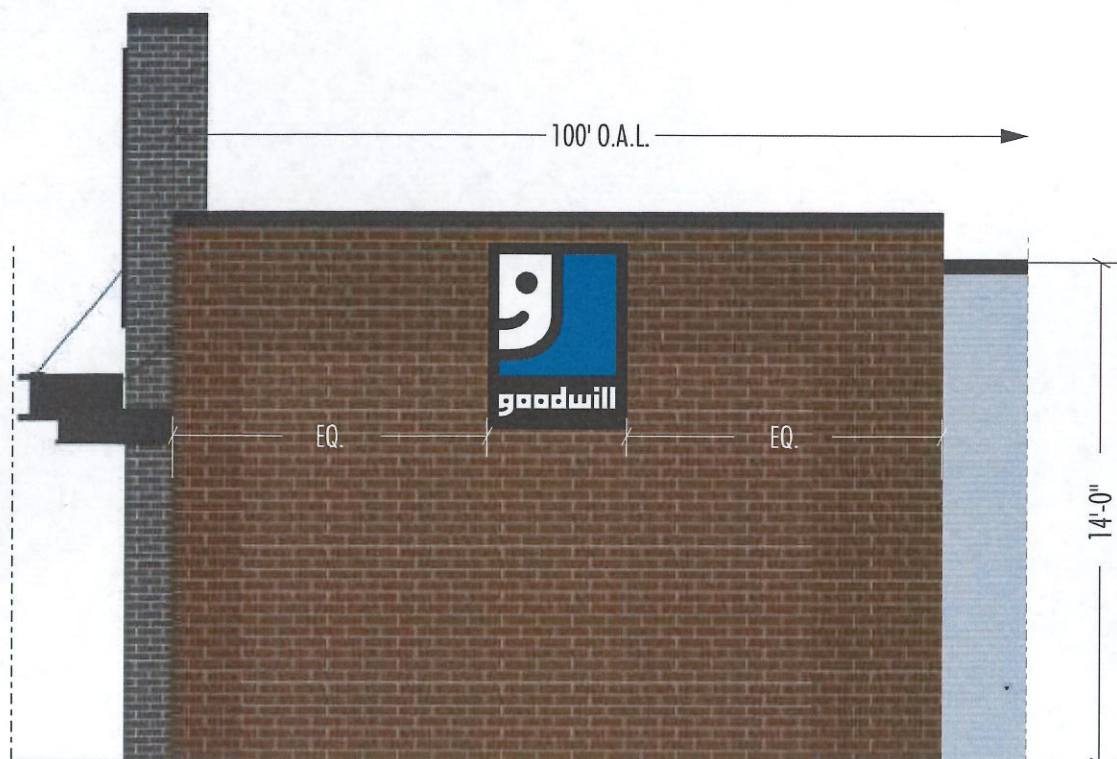
PROPOSED SIGN INSTALLATION - WEST ELEVATION
