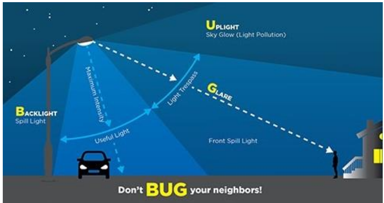
Figure IV-1: (Image credit: City of Fort Collins, CO)
