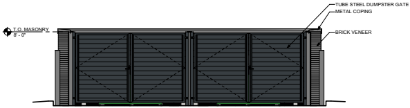
5 ELEVATION - DUMPSTER ENCLOSURE 1/4" = 1'-0"
