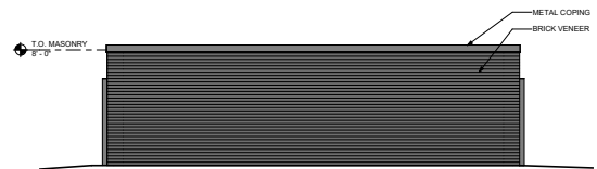
4 ELEVATION - DUMPSTER ENCLOSURE 1/4" = 1'-0"
