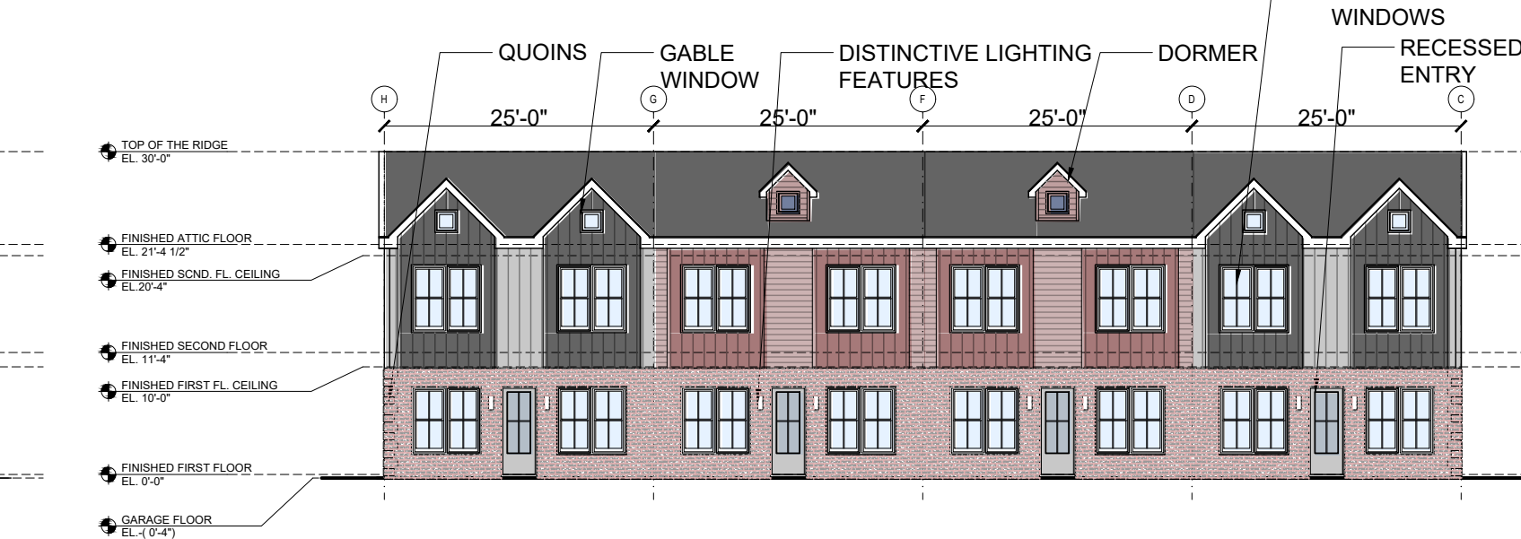
3 Building 4 East Elevation A2.00 SCALE: 1/16" = 1'-0"
