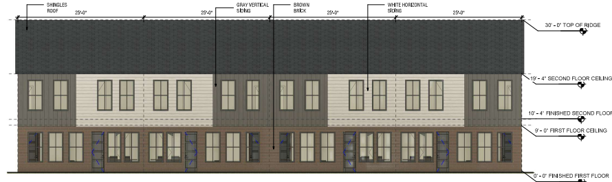
2 UNIT 1 ELEVATION - BACK 1/8" = 1'-0"
