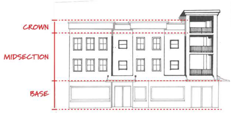
FIGURE 9.2 TRIPARTITE (3-PART) FAÇADE DESIGN
