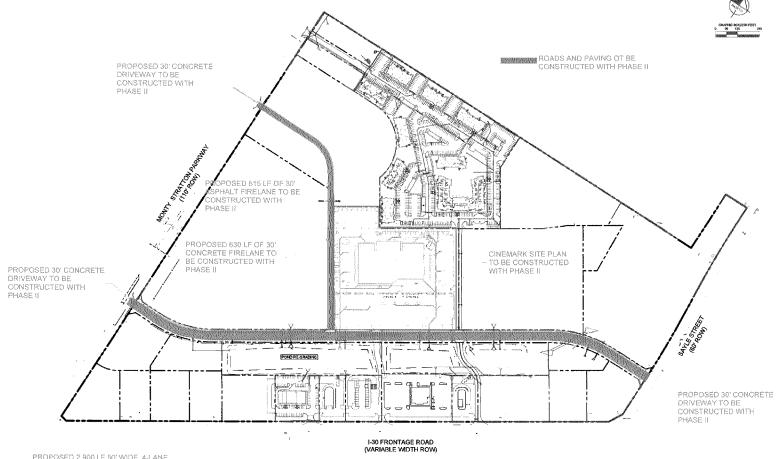
PROPOSED 2,980 LF 50' WIDE, 4-LANE PUBLIC ROADWAY (KB BLVD) INCLUDING ELECTRICAL AND LIGHTING TO BE CONSTRUCTED WITH PHASE II
