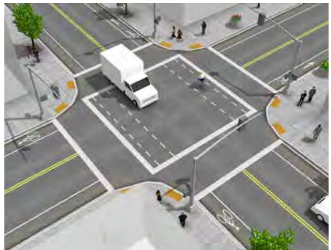
Bike Lane Intersection Markings - design credit: NACTO
