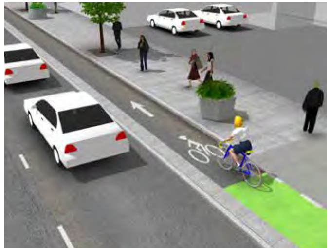
Cycle Track Intersection - design credit: NACTO
