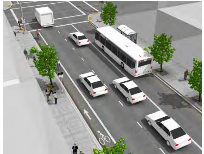
One Way Cycle Track - design credit: NACTO
