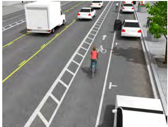
Buffered Bike Lane - design credit: NACTO
