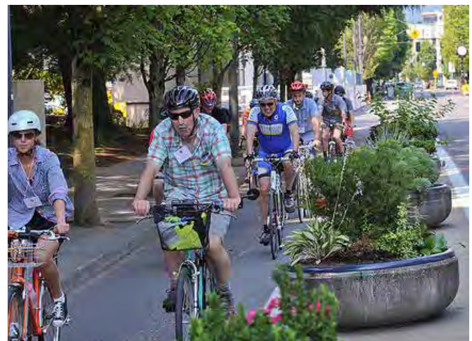
Two Way Cycle Track - Bike lanes protected by planters. Photo credit: Bike Portland
