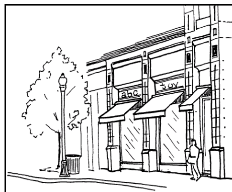
Figure 50.05.004-D: Break in Awning or Canopy Construction
