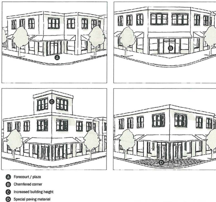
Figure 50.05.004-Q: Building Design at Street Corners
