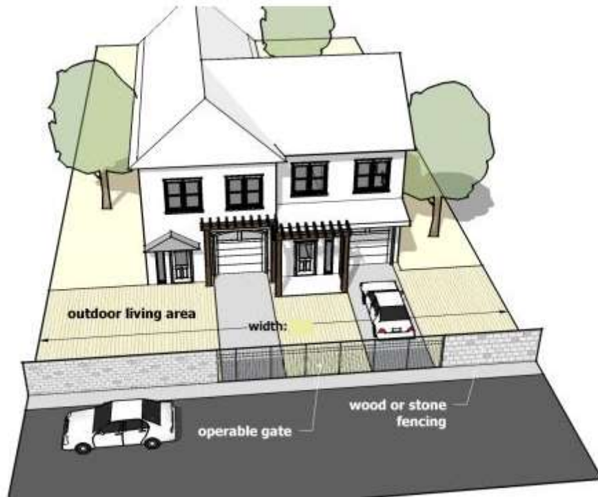
Figure 50.06.001-L: Garage Design Requirements
