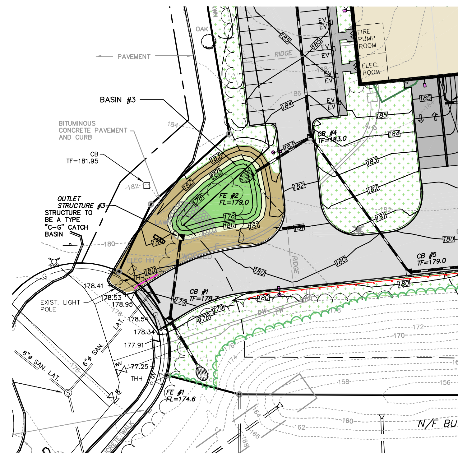
WATER QUALITY BASIN #2
