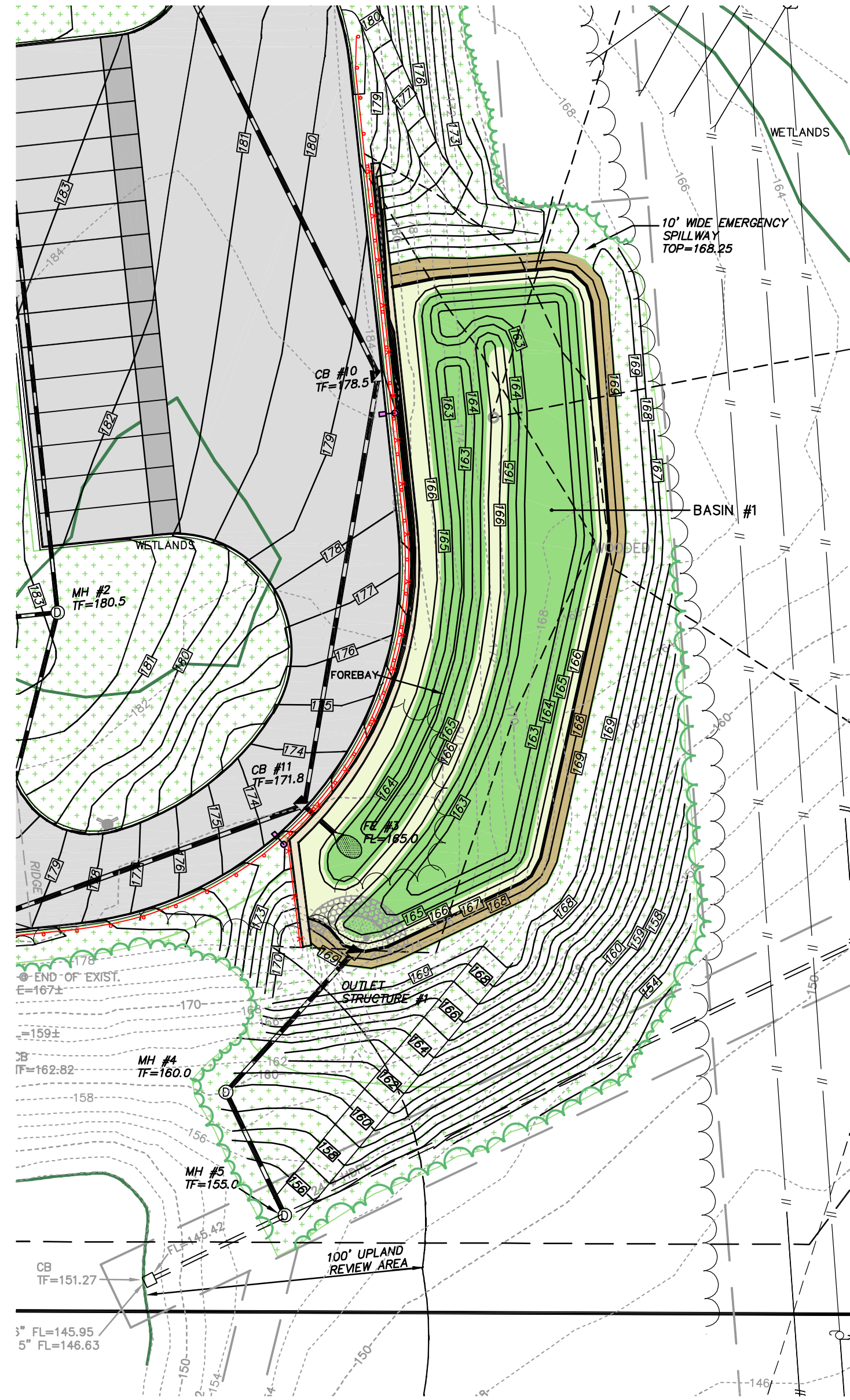
WATER QUALITY BASIN #1
