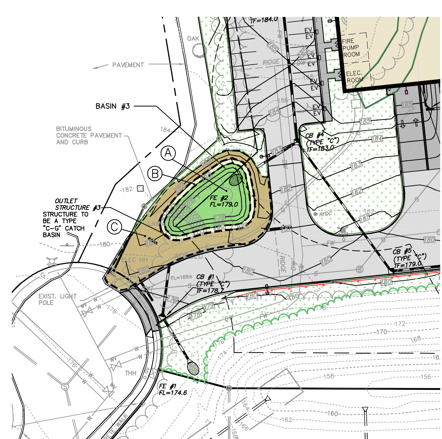
WATER QUALITY BASIN #3
