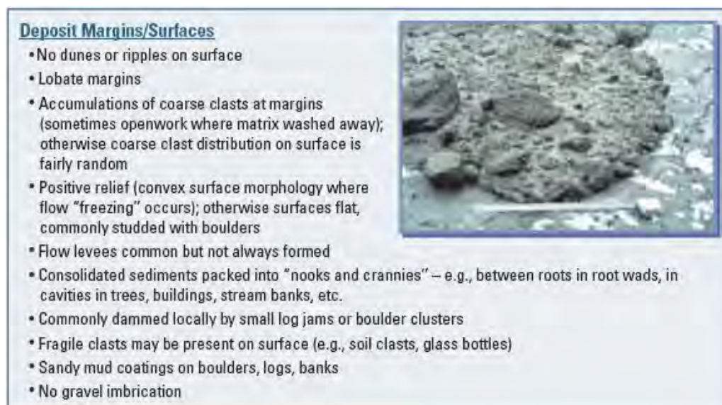
Figure 4-38 Field Evidence of Debris Flow
