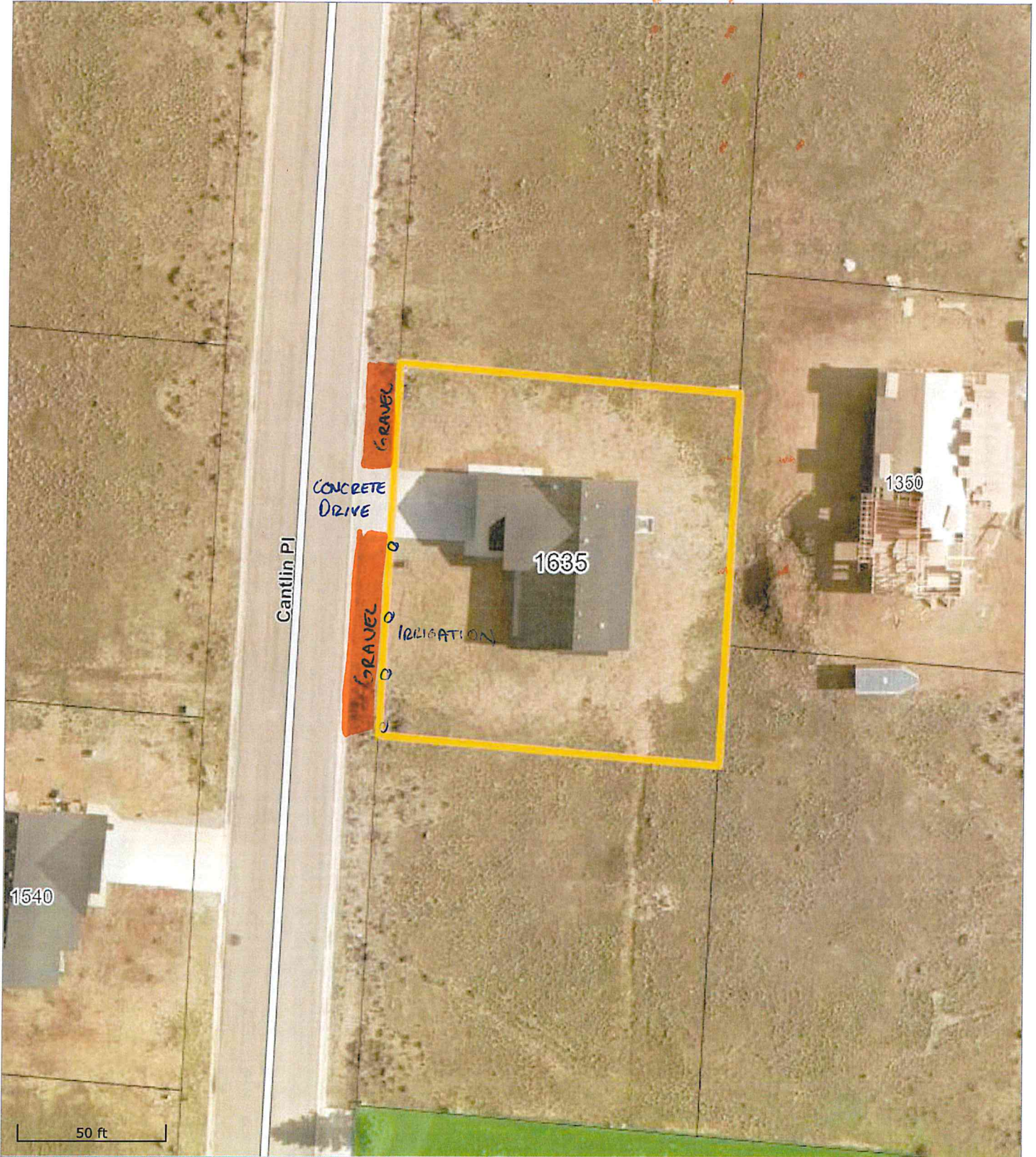
Exhibit A: 1635 Cantlin PI Install Loose Gravel and concrete driveway. Gravel to be placed below level of valleypan. Concrete Driveway to match grade of back of valleypan.
