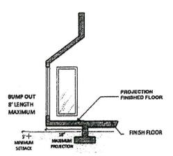
3. In corner lot yards, with 2 front yards, projections shall be permitted in 2 yards only. If placed within the front or rear yard such projection shall encroach in said yard no more than 18" in depth, be a minimum of 12" in depth, not exceed 8 feet in length, and be separated by 7 feet. If placed in the side yard such projections shall comply with section 2 above. All measurements herein shall be as measured on the exterior of the structure.
