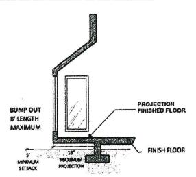
3. In corner lot yards, with two (2) front yards, where the yards are six feet six inches (6'6") or greater in width, projections shall be permitted up to eighteen inches (18") in depth and eight feet (8') in length. Projections shall be limited to two (2) yards where these projections are encroaching into the permitted setback. Any projections must be separated by seven feet (7'). All measurements herein shall be as measured on the exterior of the structure.
