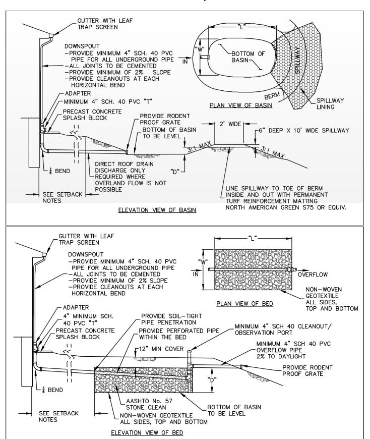
NOTE 1: Infiltration trenches may only be used for structures; infiltration basins may be used for all surfaces, including structures.
