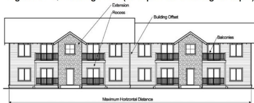
Figure 4.7-Q Building Form (Multiple unit housing example)
