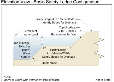
B. Safety Ledge Illustration Elevation View –Basin Safety Ledge Configuration
